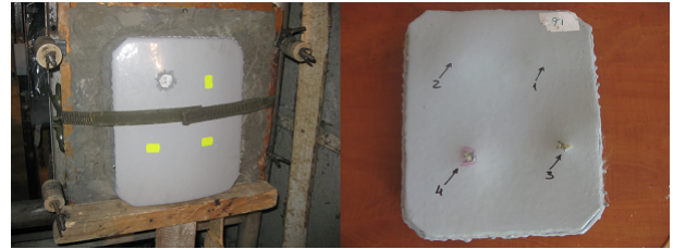
Fig. 7. Evaluation of 2.3-layered PUC3- IV level ballistic plate shot proof
